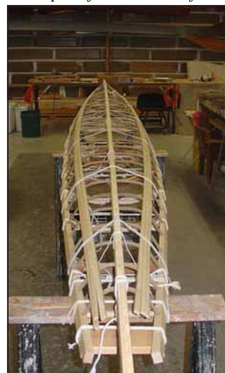
With an overall length of 18 feet, this bidarka required 31 ribs. View of hull.
