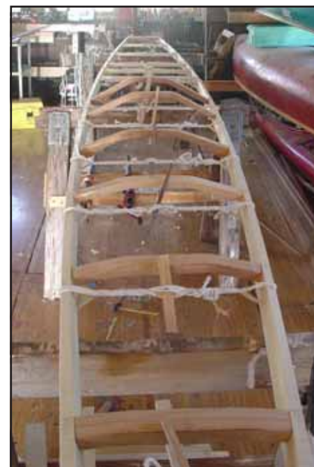
Assembly requires the use of temporary lashings to hold the gunwales and deck braces together during construction. View of boat deck looking from the bow.
