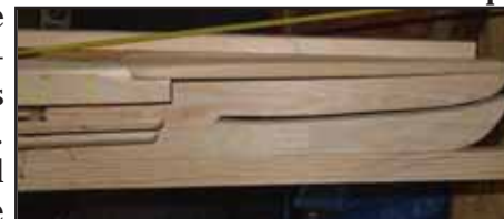
Two vertical "jaws" create a bifurcated bow unique to the bidarka. This feature when covered in fabric and stitched, creates a knife-like bow
