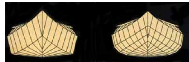
The Greenland kayak (left) with its hard chine hull design is more maneuverable but with less cargo space than the soft chine Aleutian bidarka (right). Softer chine results in a more rounded hull shape.
