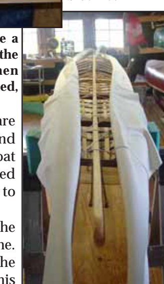
Fabric is wrapped around the hull and laced tight.
